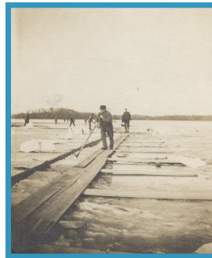
Men standing on the narrow wooden boardwalk cutting blocks of ice by hand.
